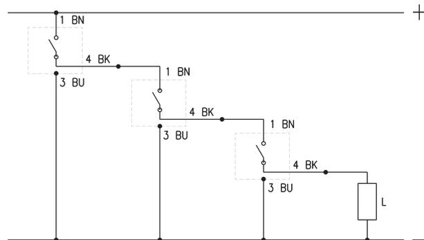
**Magnetic proximity switches with 2- or 3-wire cable for T-slot**
