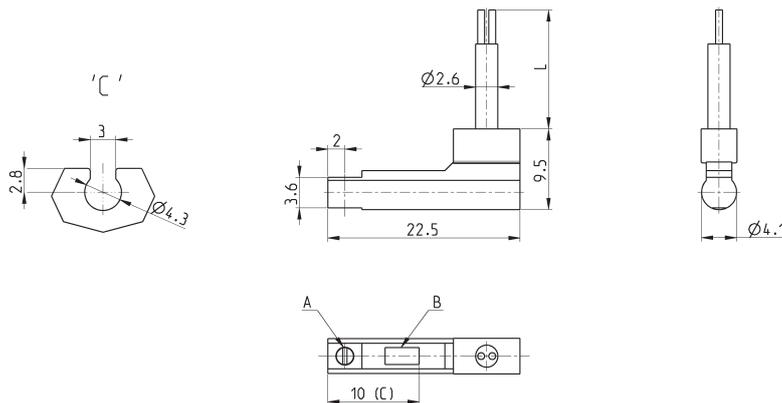
In case of polarity reversing the sensor will still be operating, but the LED diode won't turn on.
