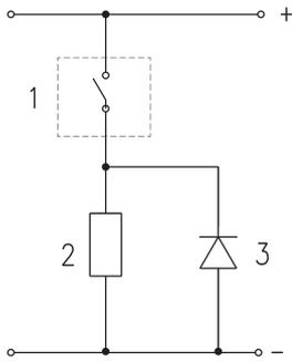
DC applications: there is no protection on the Reed sensors on the inductive load, therefore it is advisable to use an electric circuit with protection against the voltage spikes. See picture above for a typical example.
