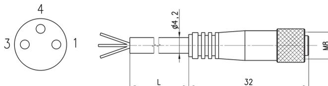
In case 2-wire sensors with M8 connector (Mod. CST-250N, CSV-250N, CSH-253) are used, please connect the brown wire to the supply (+) and the black wire to the load.
