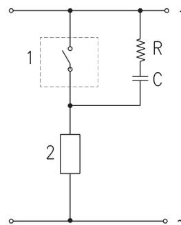
AC applications: there is no protection on the Reed sensors on the inductive load, therefore it is advisable to use an electric circuit with protection against the voltage spikes. See picture above for a typical example.
