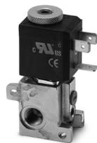
The 3/2-way solenoid valves for manifold assembly are available in the NC and NO in line version, with G1/8 ports at the manifold inlet. The inlets can be with M5 threading or with a Ø 4 cartridge.
