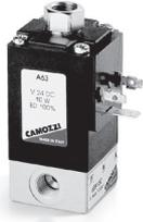
In the mod. 648-150-A6\* (NO) connections 1 and 3 are inverted, while the max operating pressure is 6 bar in case a solenoid A6B, A6C, A6D, A6E is chosen.
