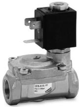
The pilot of these indirectly operated solenoid valves controls the diaphragm position through a differential pressure. These valves are therefore particularly suitable for controlling high fluid flow rates and require very low working pressures.
