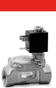
The pilot of these indirectly operated solenoid valves controls the diaphragm position through a differential pressure. These valves are therefore particularly suitable for controlling high fluid flow rates and require very low working pressures. Ports: from G3/8 to G2.
