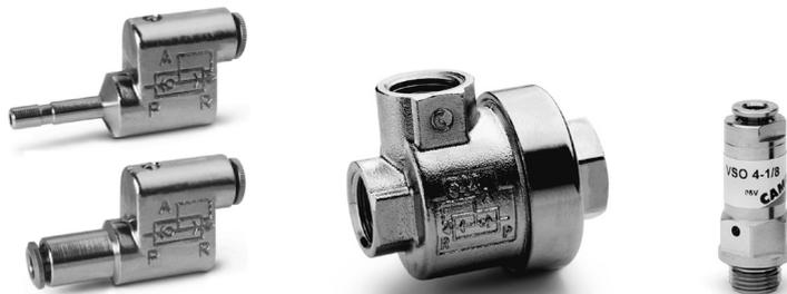
**Series VSC and VSO quick exhaust valves are commonly used to increase the speed of cylinders or for rapid depressurisation of tanks containing compressed air.**
