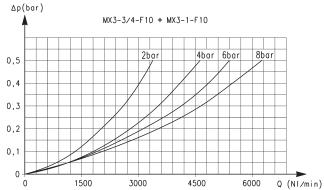
Reference diagram for models with filtering element = 25  $\mu m$
